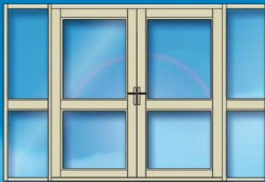
Double Hinged Front Entry Door and two Sidelites, all with Midrails
